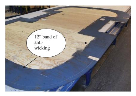
**Airstream also** applies additional moisture protection around the perimeter and edges of the flooring using a 12" band of anti-wicking material. It is manufactured by Dolphin adhesives.
